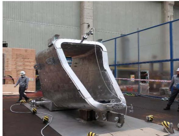
Factory Acceptance Test (Pressure Test) of LPSE 10
