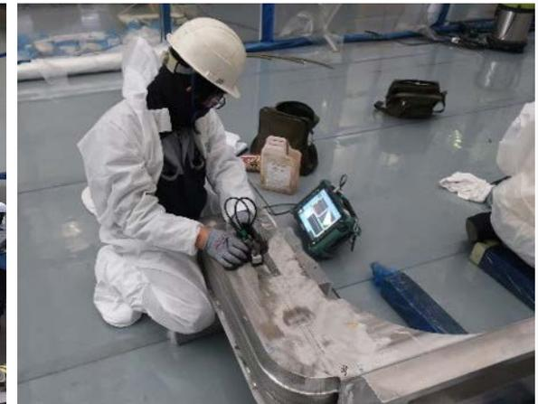
Phased Array UT (NDE) inspection on Shield Plate weldment of NB PSE
